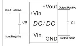
②Input reflecting ripple current test circuit:
